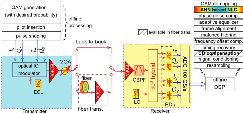
Fig. 4: Experimental setup for a dual polarization probabilistically-shaped 28 GBaud 64/256-QAM systems. ECL: external cavity laser, EDFA: Erbium-doped fiber amplifier, VOA: variable optical attenuator, OBPF: optical bandpass filter, LO: local oscillator, PDs: photodetectors, CD: chromatic dispersion, DSP: digital signal processing, ANN-based NLC: artificial-neural-network based nonlinearity compensation, trans.: transmission.
