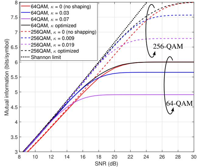
Fig. 1: Comparison in terms of mutual information between 64-QAM and 256-QAM under different shaping factors. Note that  $\kappa = 0$  means uniform constellation (no shaping).
