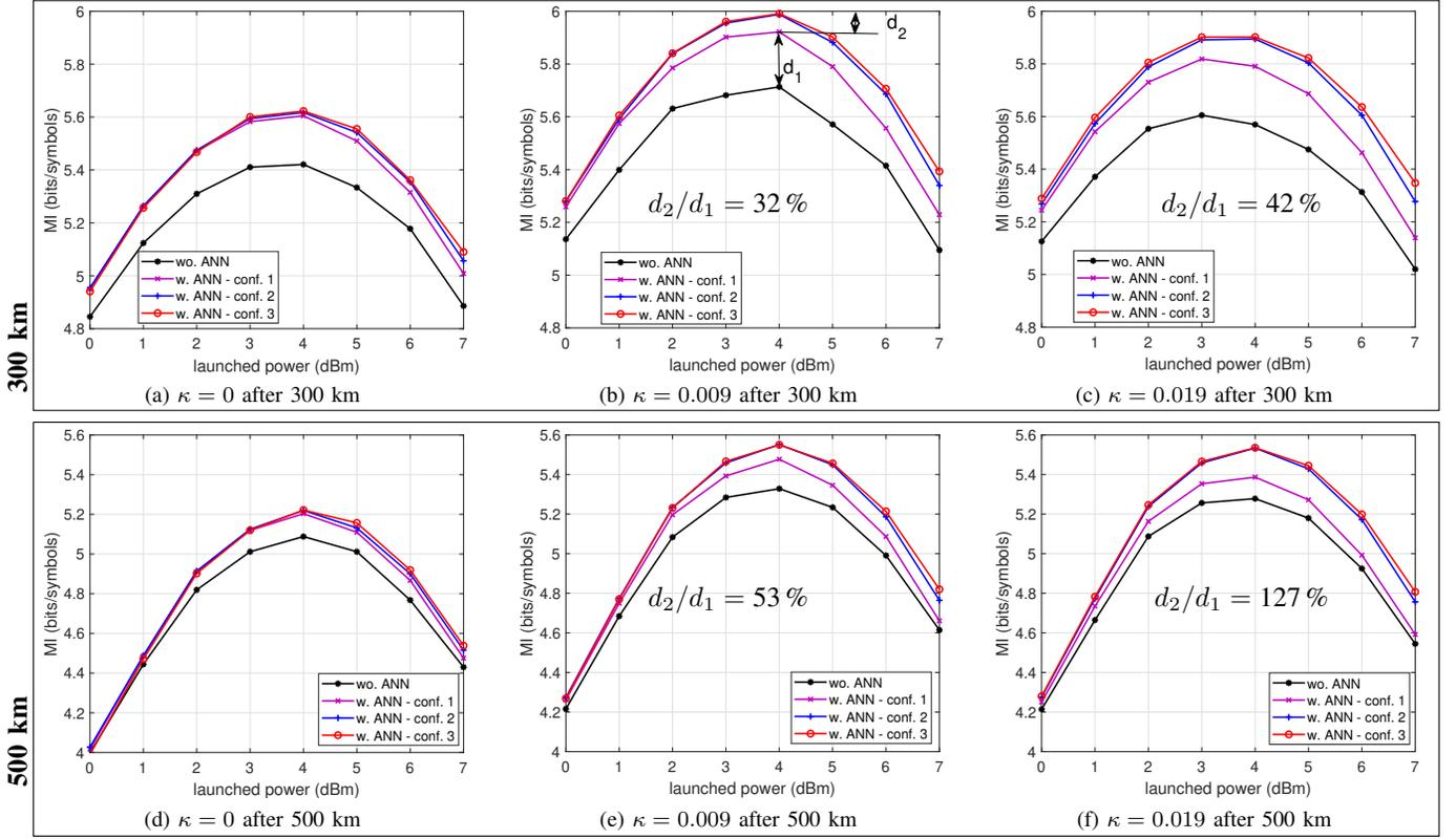
Fig. 6: Performance of the proposed ANN-based NLC for PS DP 256-QAM systems after 300 km and 500 km of fiber transmissions with different ANN configurations. (a) uniform constellation after 300 km, (b) PCS with  $\kappa = 0.009$  after 300 km, (c) PCS with  $\kappa = 0.019$  after 300 km, (d) uniform constellation after 500 km, (e) PCS with  $\kappa = 0.009$  after 500 km and (f) PCS with  $\kappa = 0.019$  after 500 km.
