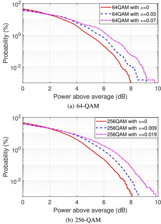
Fig. 2: PAPR comparison of QAM signals under different shaping rates: (a) 64-QAM and (b) 256-QAM.
