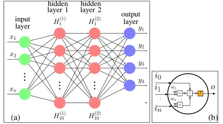
Fig. 3: (a) Structure of artificial-neural-network-based nonlinear compensation (ANN-based NLC). (b) Input-output relationship of a “neuron” in the hidden and output layer.
